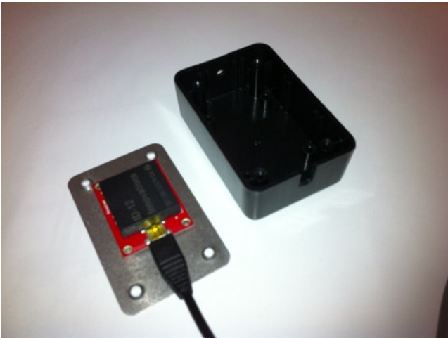
Figure 9-7. Assembling the RFID reader unit
