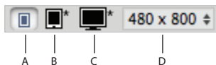
A. Mobile size (480 × 800). B. Tablet size (768 × 1024). C. Desktop size (1000w). D. Window Size.
